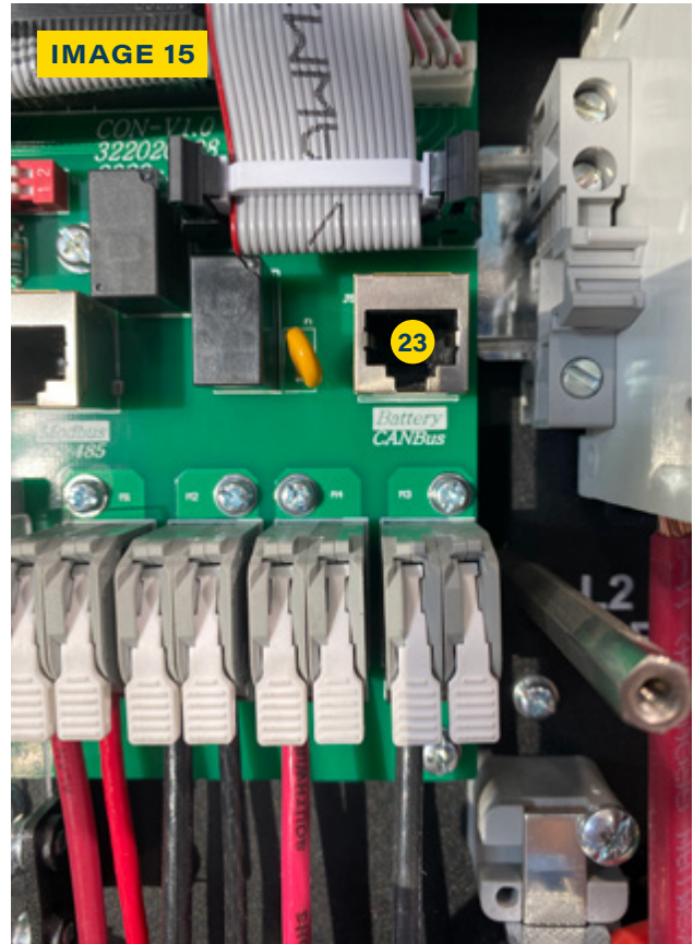
23 CANBUS PORT ON SOL-ARK INVERTER.
