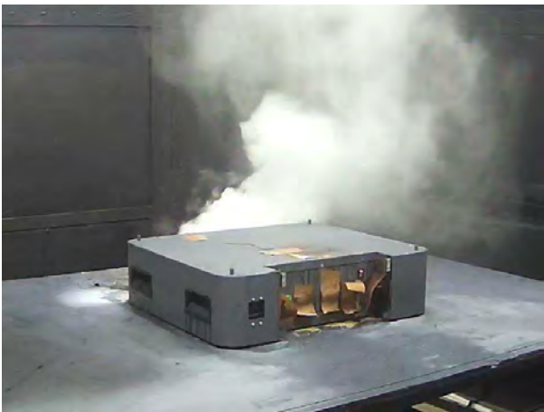
(k) Thermal runaway of other cells [02:28:42]
