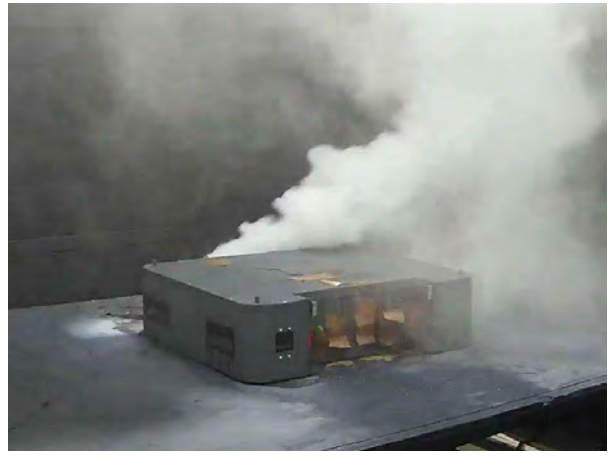
(j) Thermal runaway of adjacent cell 11 [02:27:20]
