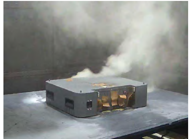
(h) Thermal runaway of adjacent cell 07 [02:21:20]
