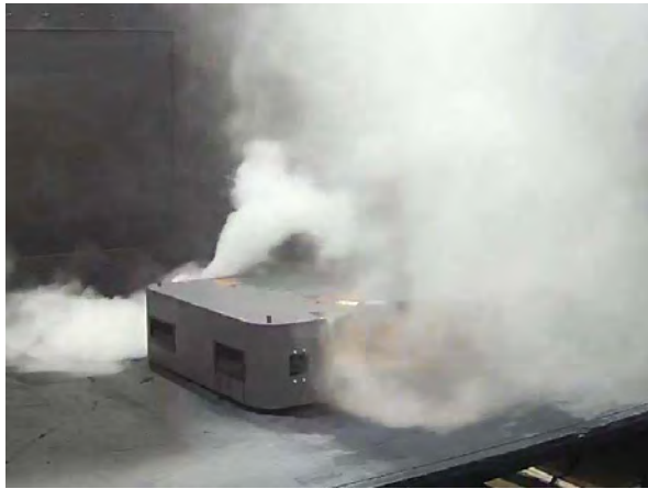
(g) Thermal runaway of adjacent cell 13 [01:01:07]
