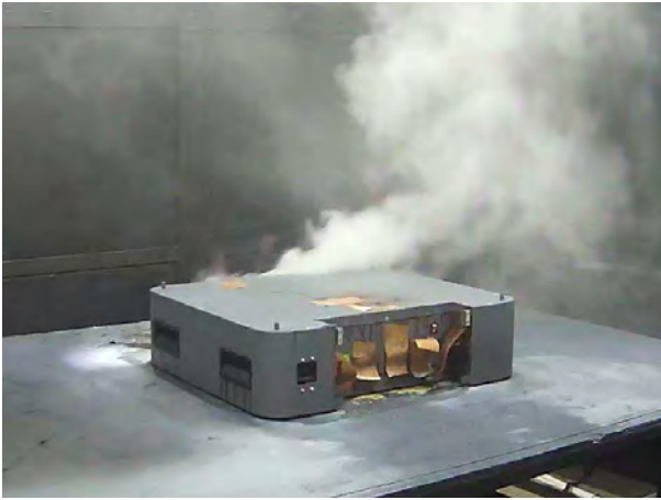
(i) Thermal runaway of adjacent cell 10 [02:24:53]
