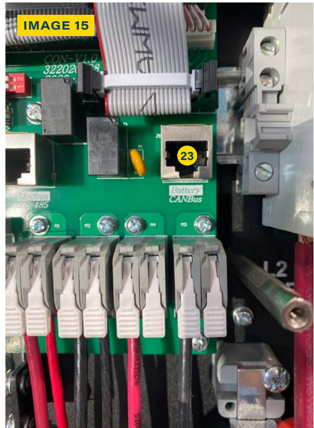
23 CANBUS PORT ON SOL-ARK INVERTER
