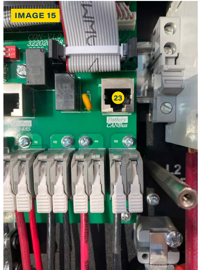
23 CANBUS PORT ON SOL-ARK INVERTER.
