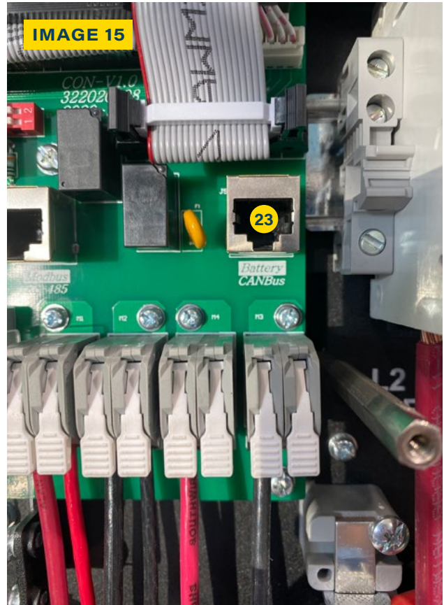
23 CANBUS PORT ON SOL-ARK INVERTER
