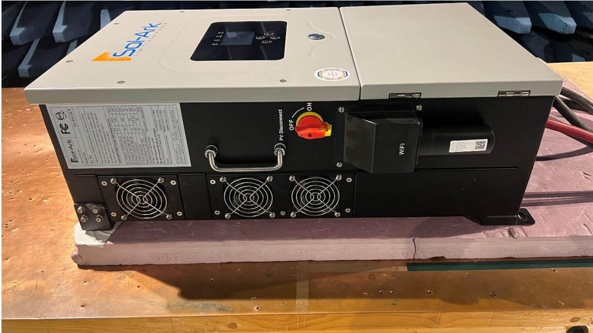
08 Support Equipment - Sol-Ark 12k-P
