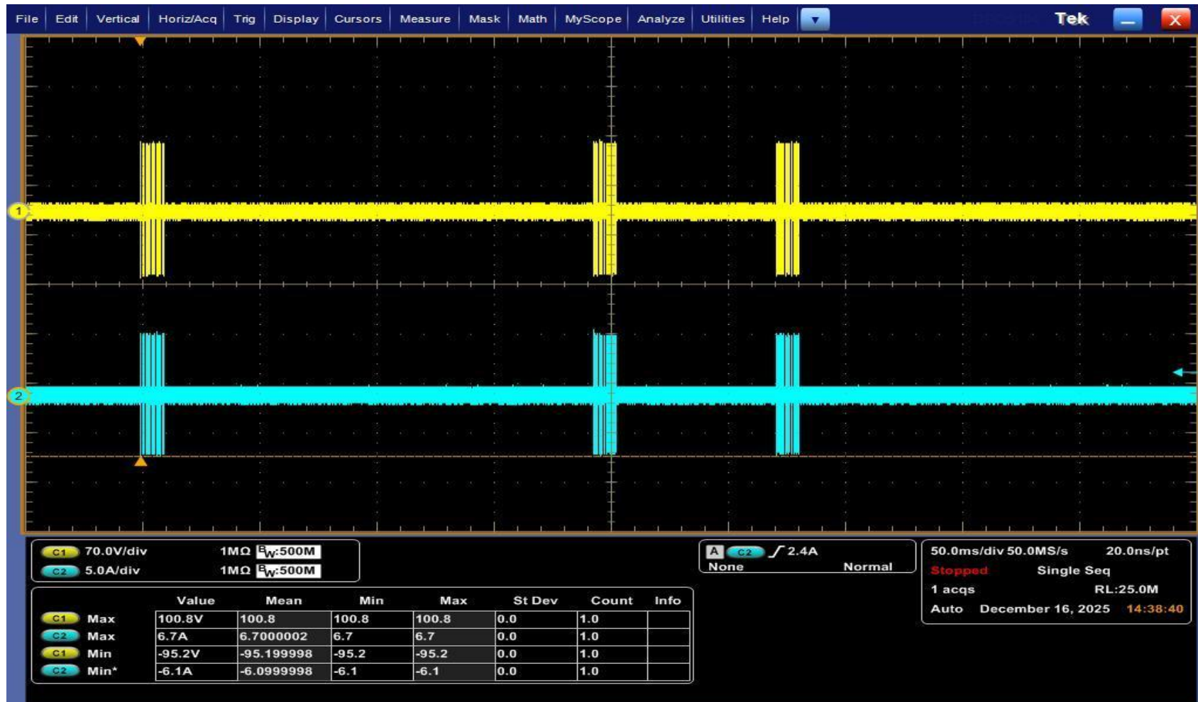
49 CS117 - Active - WF3 - 10 MHz - Positive - Multiple Burst - Power Bundle
