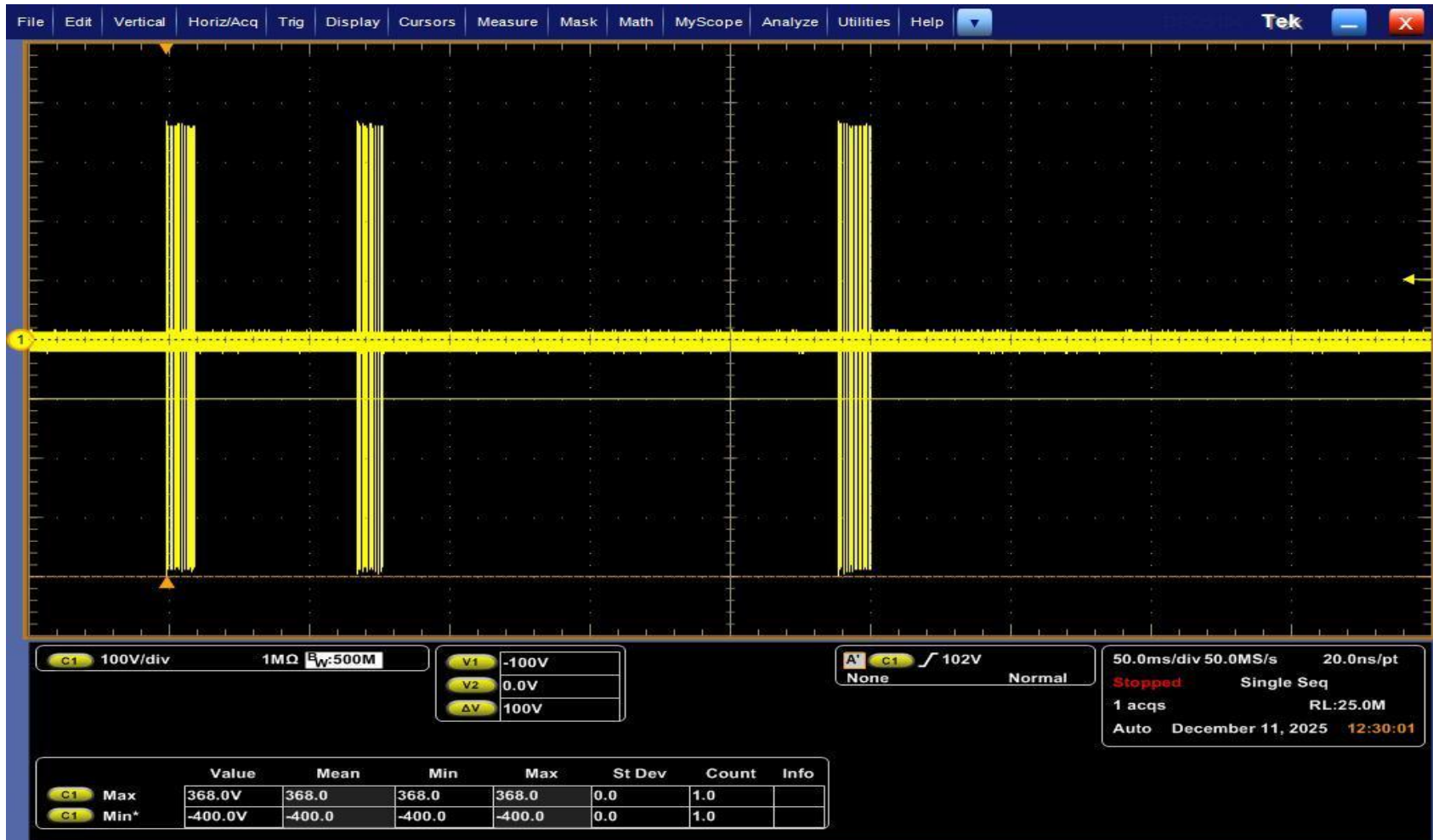
25 CS117 - Verification - WF3 - 10 MHz - Positive - Multiple Burst - Burst Application
