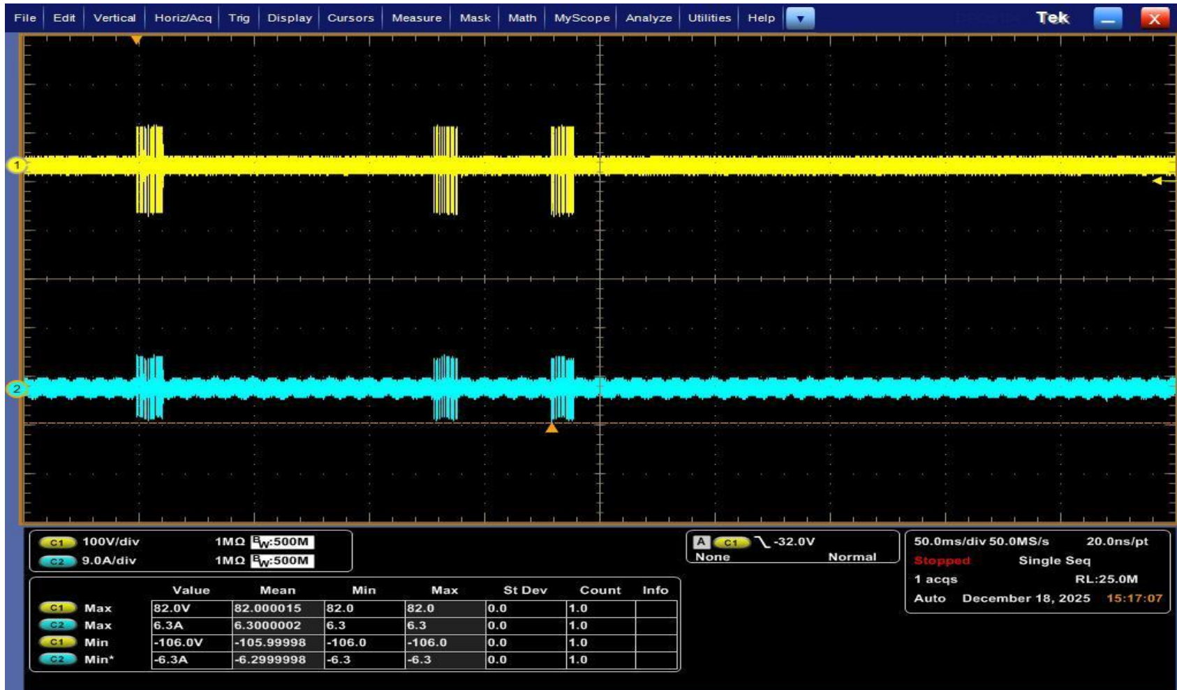
44 CS117 - Active - WF3 - 1 MHz - Negative - Multiple Burst - High Side
