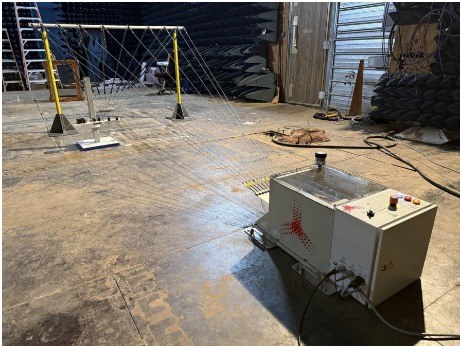
02 RS105 - Verification Setup
