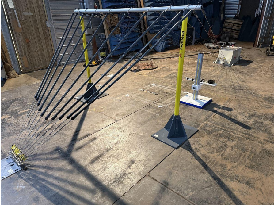
01 RS105 - Verification Setup
